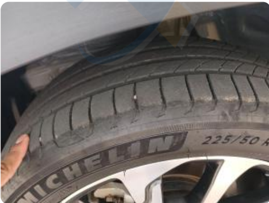
(L) Front Tyre - Crack, Cut
